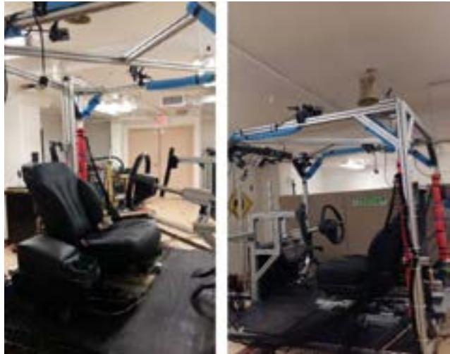
A custom sled apparatus exposed subjects to low-severity, non-injurious loading conditions that mimic pre-crash swerving events.
