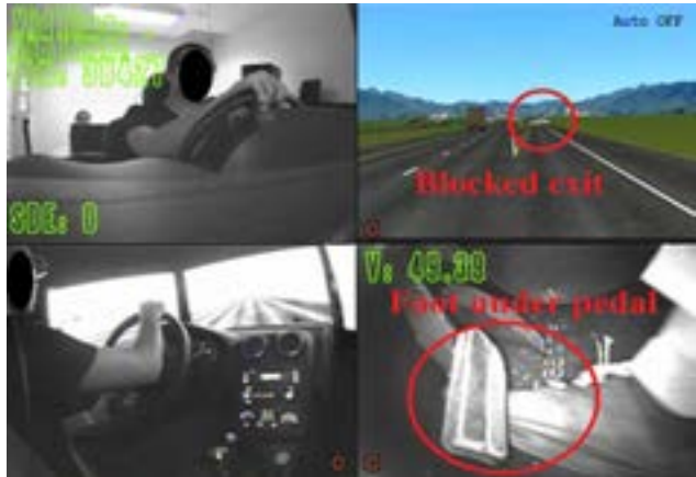
The Realtime Technologies, Inc. HD self-driving simulator in automatic mode: The upper and lower left quadrants show a study participant in the driving simulator; the upper right quadrant shows an emergency situation that requires the driver to react; and the lower right quadrant shows the participant’s foot under the pedal when seeing the emergency situation.
