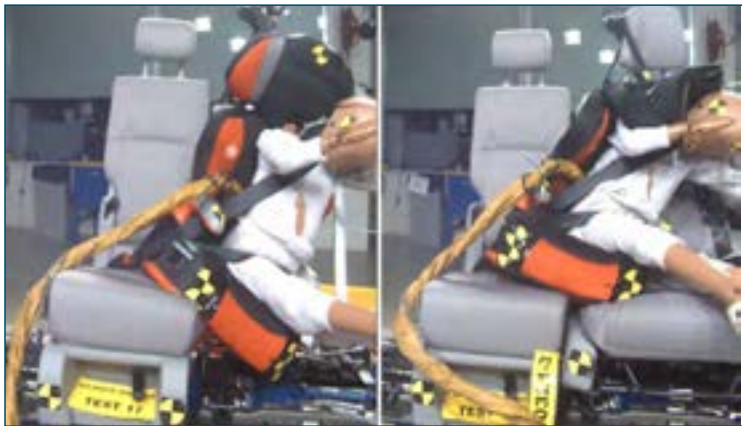
The 6-year-old Hybrid III ATD in a high back booster is installed on a narrow center seat position and exposed to a side impact when the adjacent outboard seat is removed (left) and in its standard upright position (right).
