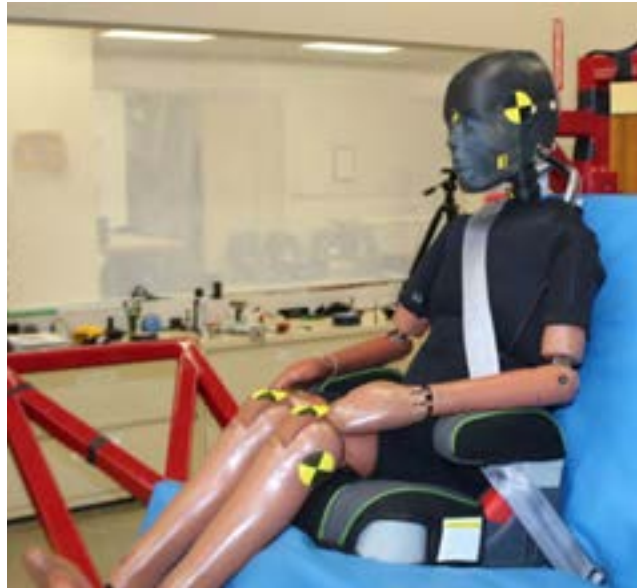
The LODC dummy representing a 10-year-old child is set up for a sled test.
