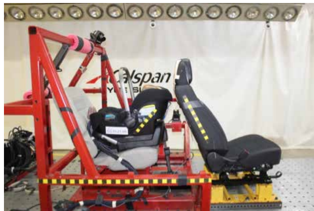
An 18-month-old ATD seated in a rear-facing infant CRS with support leg installed in the test buck.
