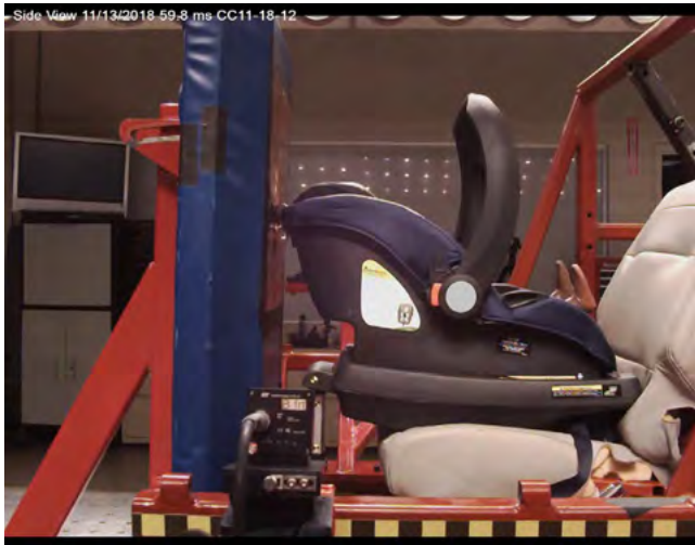
The 12-month-old CRABI ATD is tested in a RF CRS with LATCH and a load leg during a frontal impact. There was no head contact with the blocker plate.
