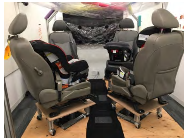
Seating fixture with seats arranged in an 'X' configuration. Front seats are rotated 135° from their usual position and rear seats are rotated 45° from their usual position. Right seats are rotated to the left and left seats are rotated to the right. All seats directly face the seat diagonally opposite itself.
